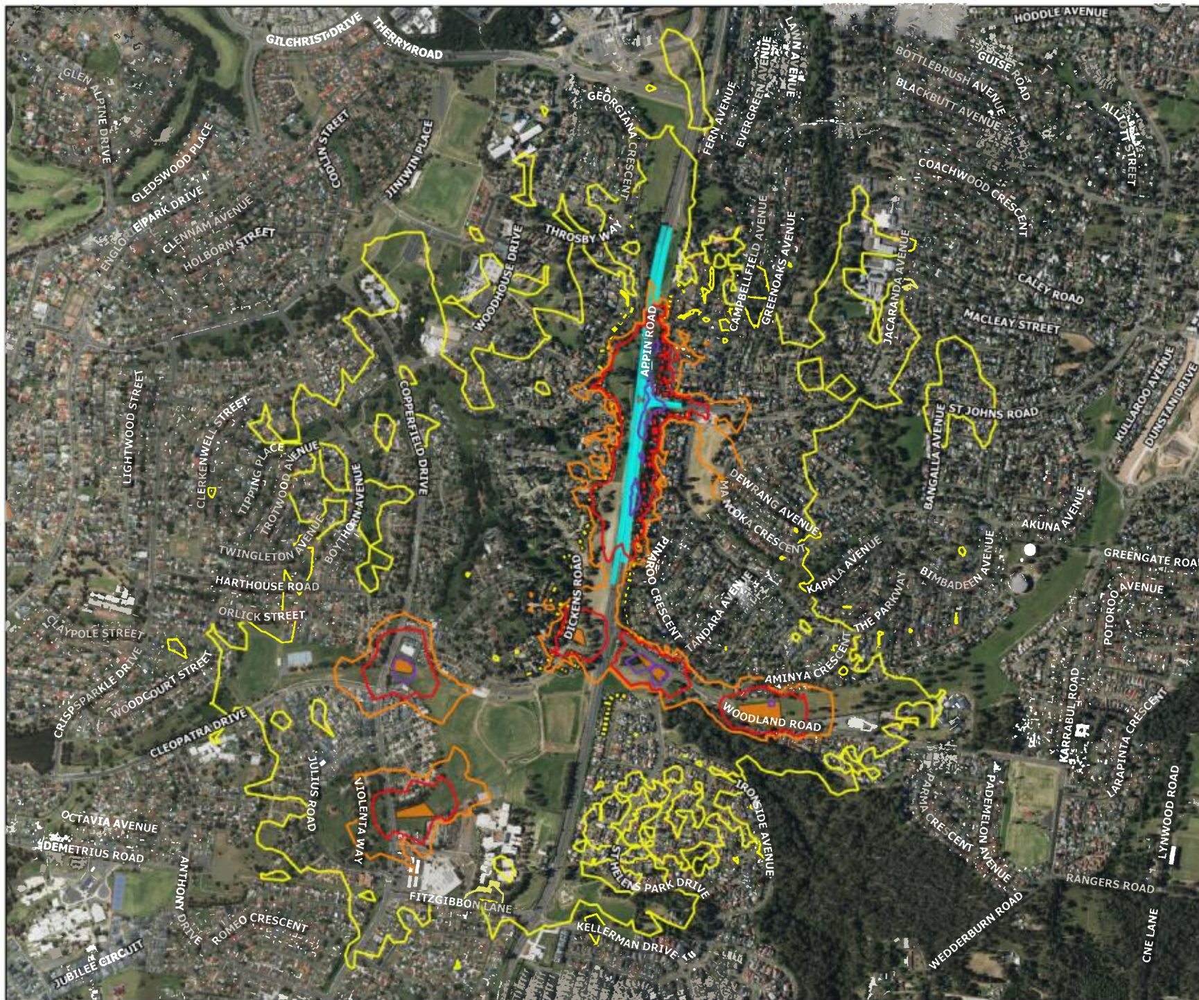
FIGURE D2 Noise Contours Corridor Clearing (S2) MAC231792-01 Appin Road Intersection
