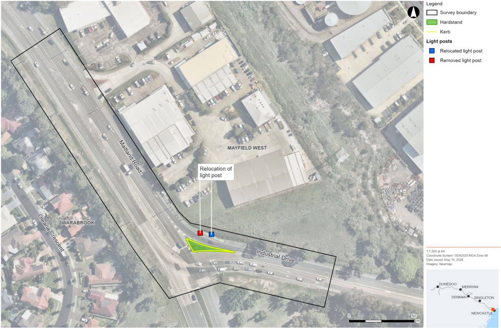
Figure 2-7: Utility impacts – Industrial Drive and Pacific Highway intersection (I-003)
