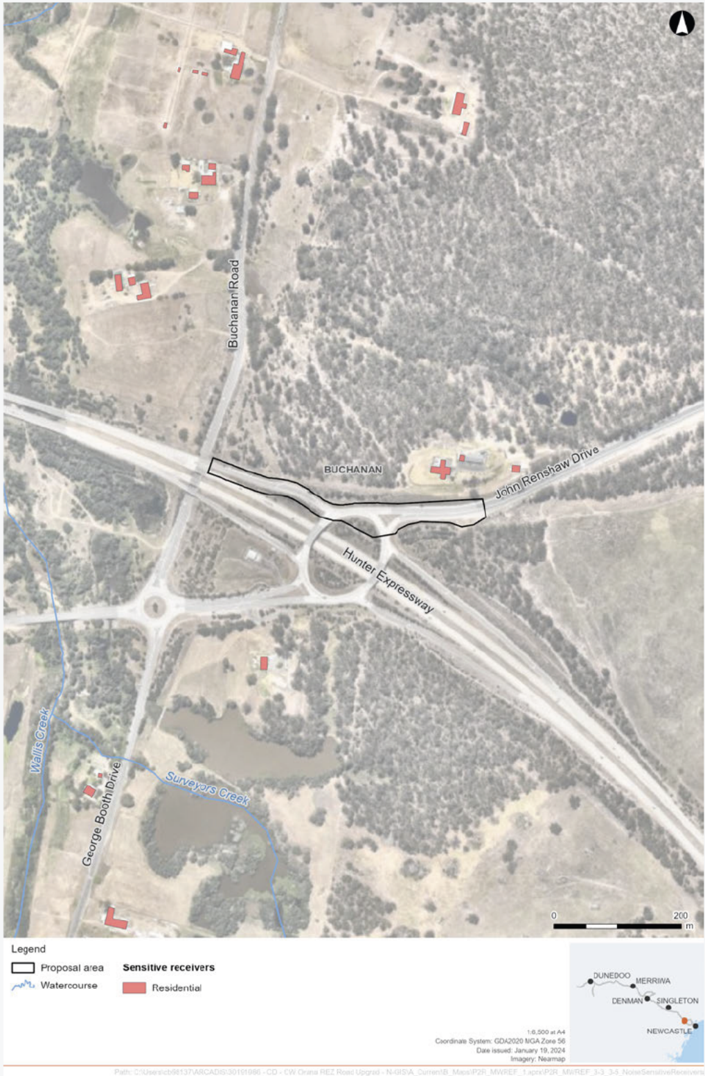
Figure 3-11: Noise sensitive receivers in proximity to the John Renshaw Drive onto Hunter Expressway Exit Ramp (I-004)
