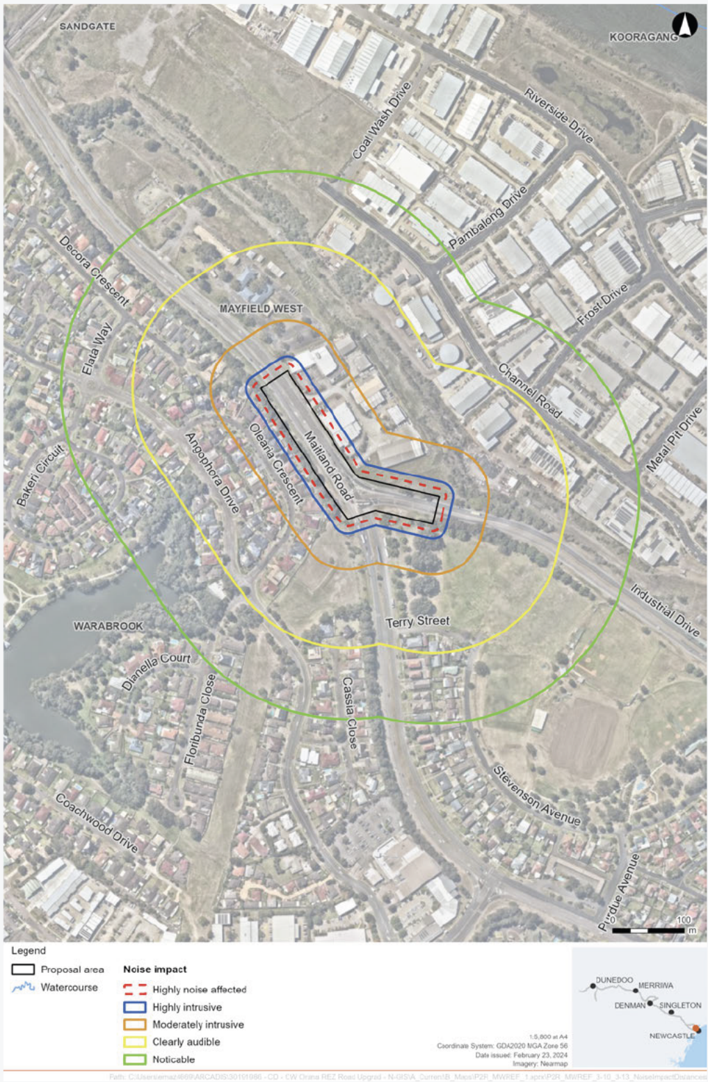
Figure 3-13: Noise impact distances during the night-time period (without line of sight) – Industrial Drive and Pacific Highway intersection (I-003)
