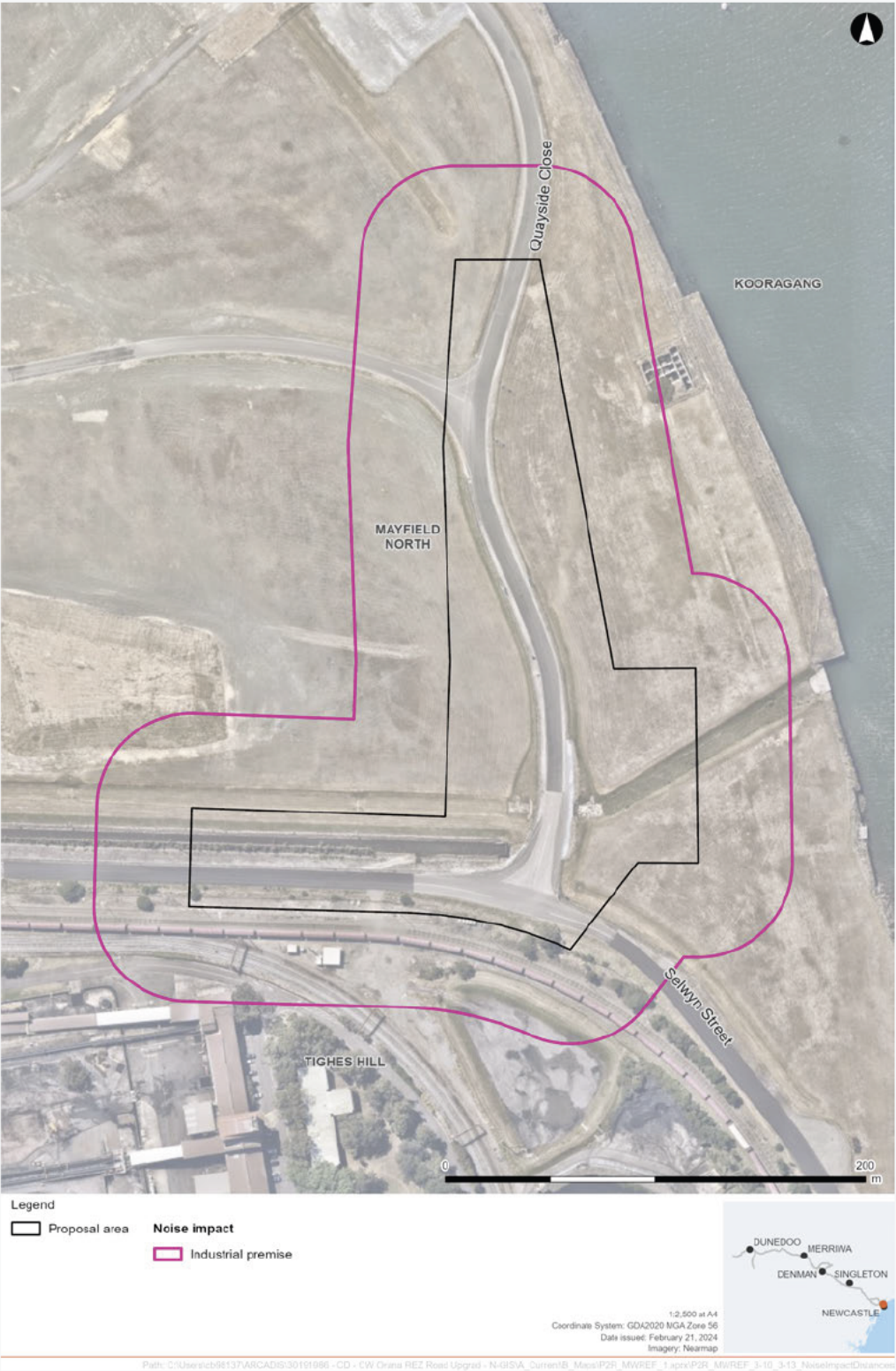
Figure 3-15: Noise impact distances during the day-time period – Quayside Close and Selwyn Street intersection (I-001)
