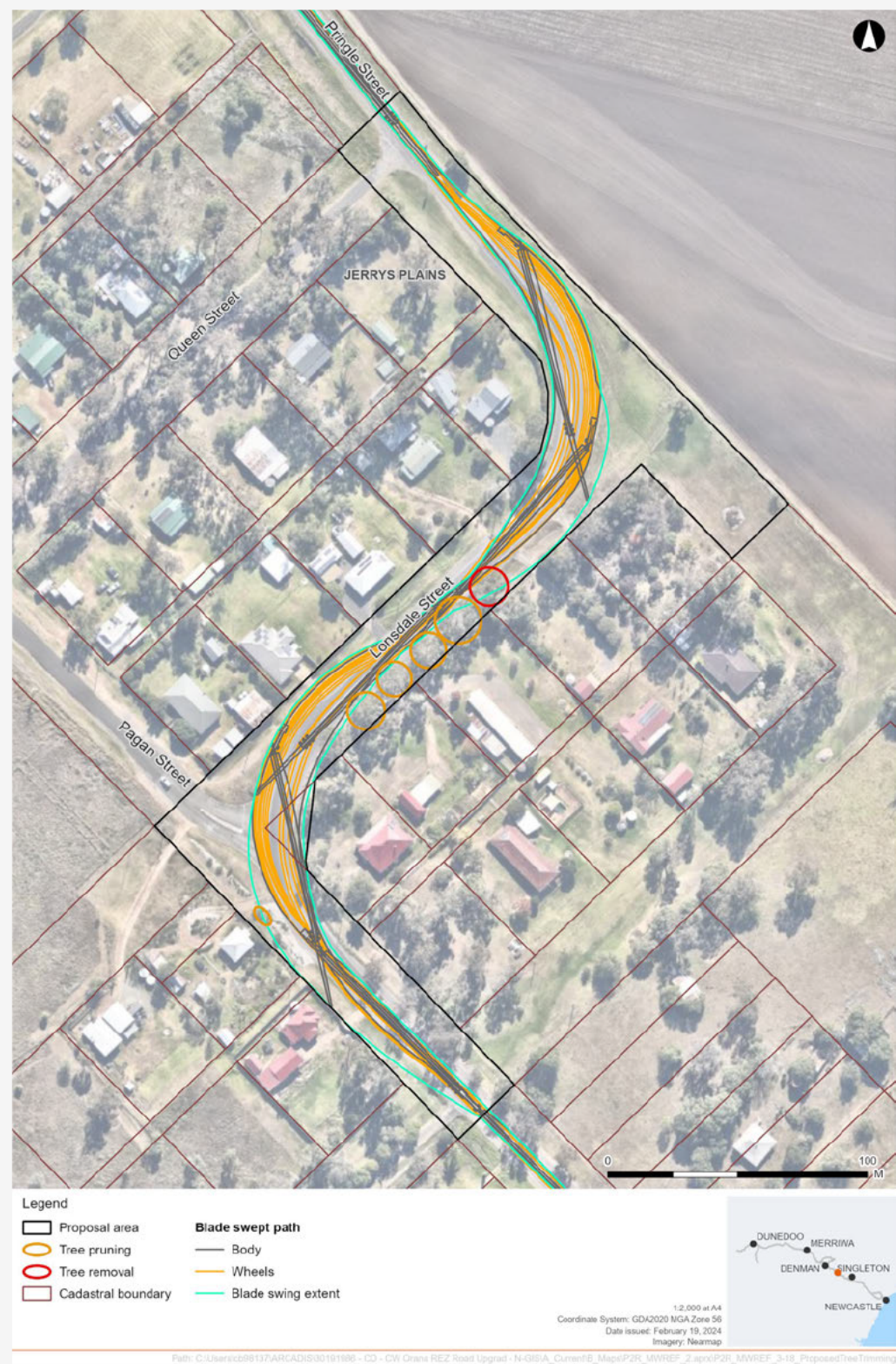
Figure 3-19: Tree removal and tree pruning requirements – Lonsdale Street and Golden Highway intersections (H-009 and H-010)
