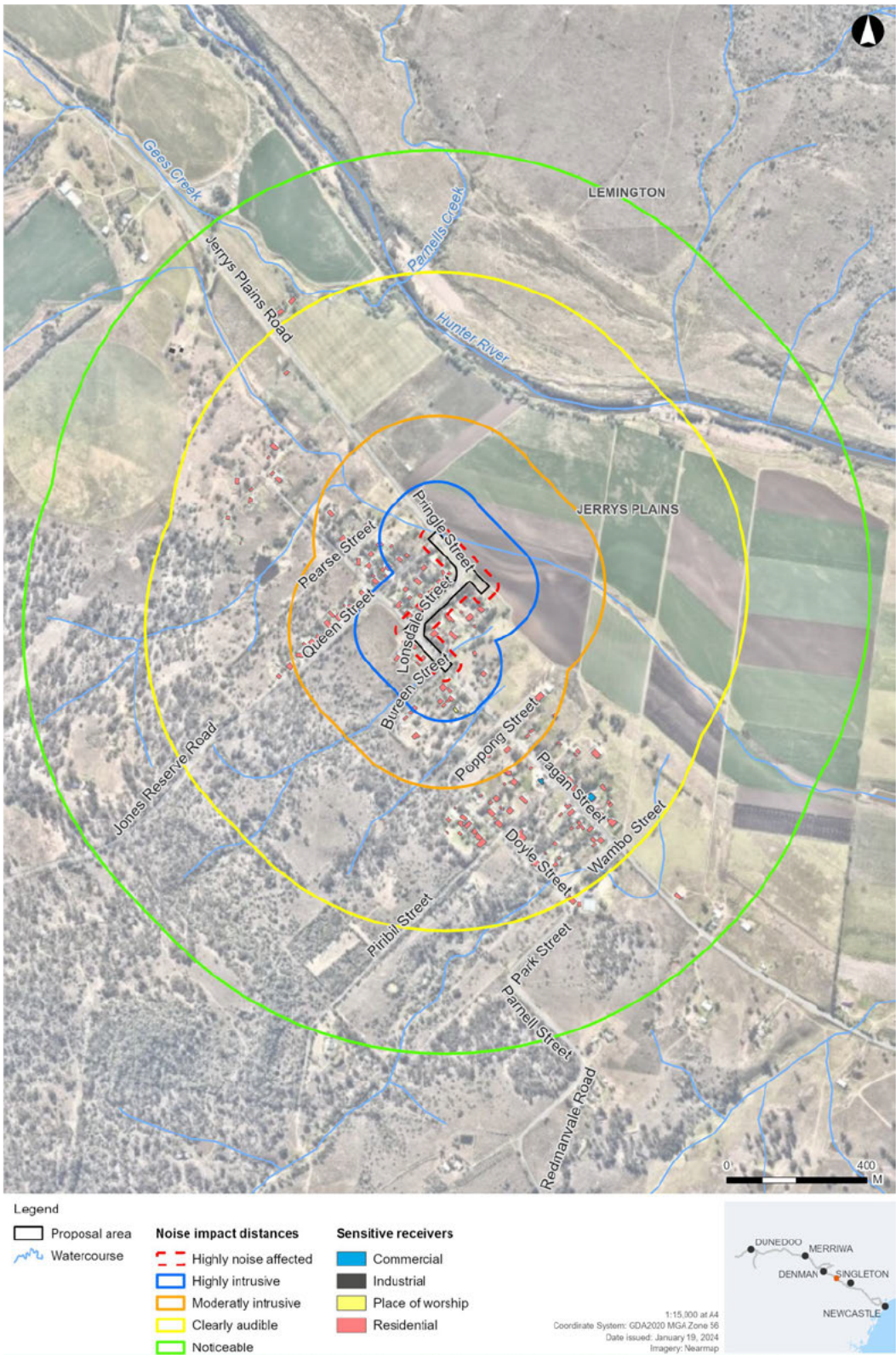
Figure 3-12: Construction noise impact distances during the night-time period (without line of sight) – Lonsdale Street and Golden Highway intersection (H-009 and H-010)
