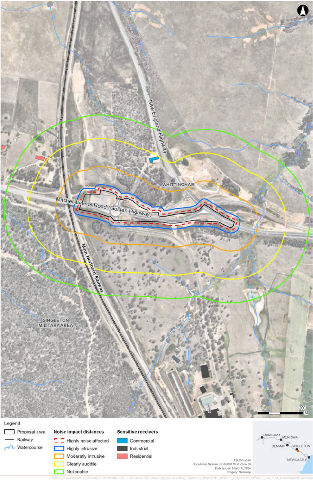
Figure 3-10: Construction noise impact distances during the night-time period (without line of sight) – New England Highway and Golden Highway intersection (I-005)
