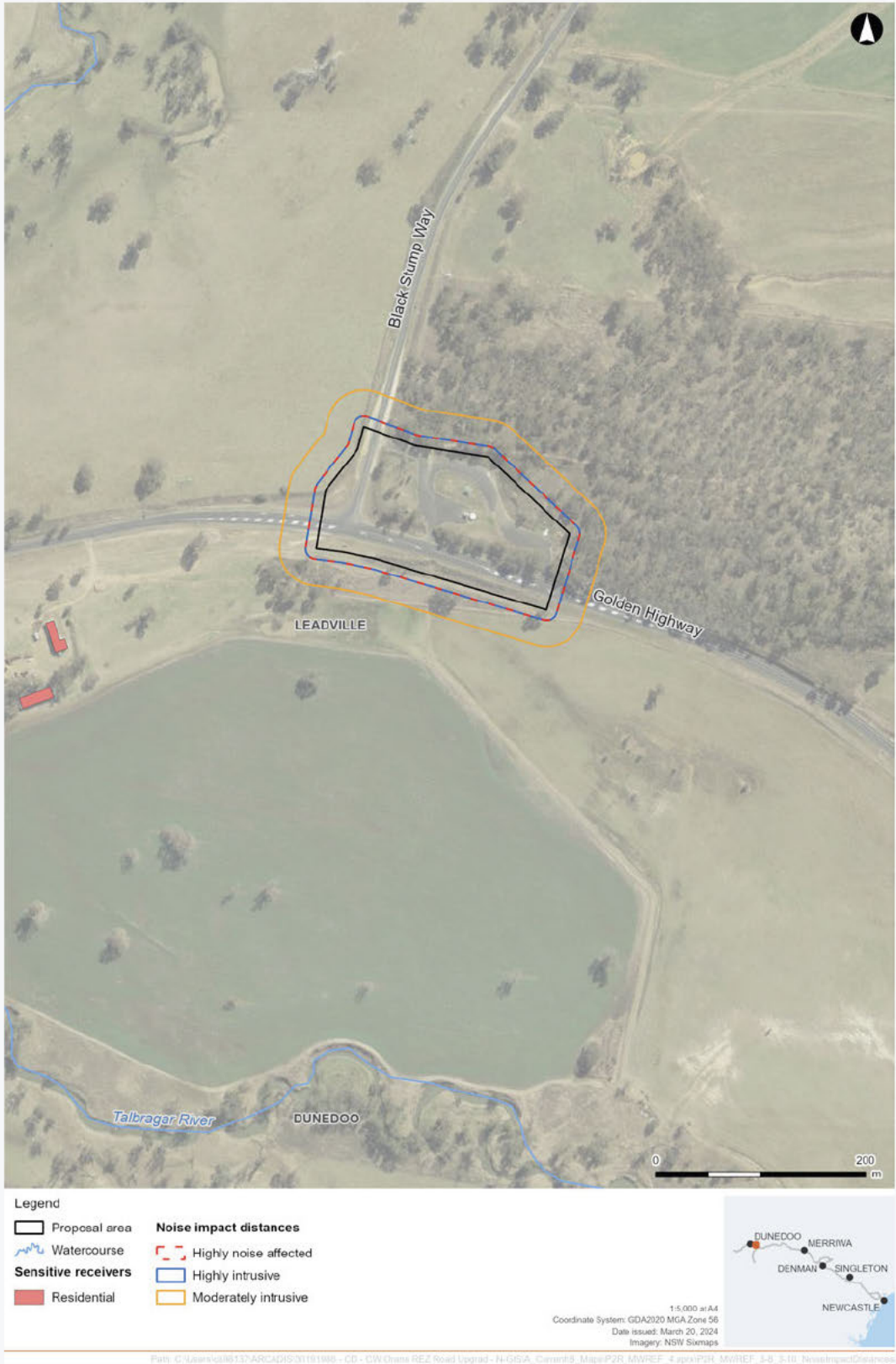
Figure 3-9: Noise impact distances during the day-time period (without line of sight) - Golden Highway and Black Stump Way intersection (I-013)
