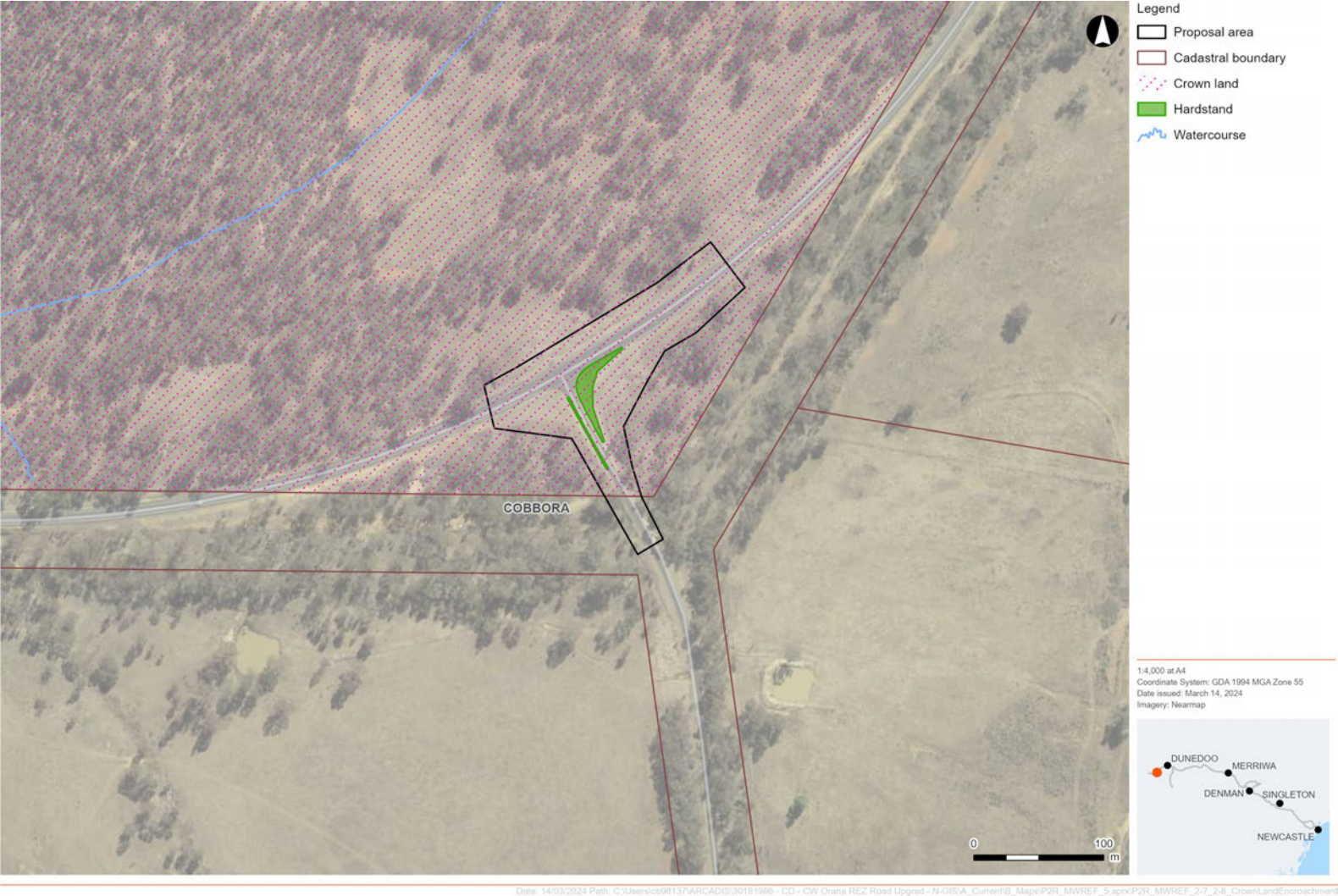
Figure 2-8: Encroachment of Crown land -Golden Highway and Spring Ridge Road intersection (I-015)
