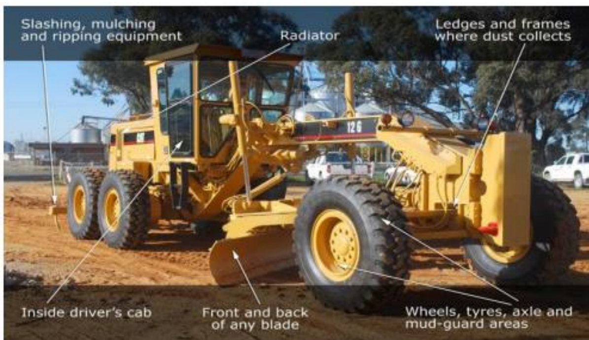
Figure 7.7: Target areas for cleaning to remove soil, seeds and plant parts (Source: EFS-33 Vehicle hygiene)
