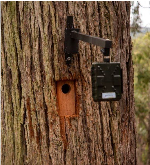
Figure 8.11: Example of remote camera installed via a bracket to monitor a carved hollow (Photo: William Terry).
