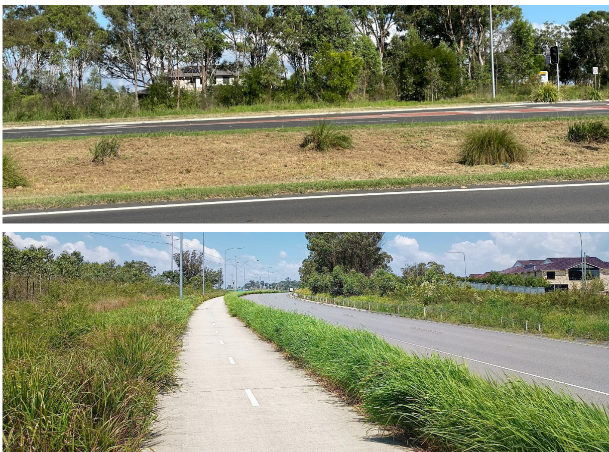
Figure 6.2: Effective early weed management during construction, and good landscape practice, can be the difference between costly ongoing management resulting in almost total plant loss (above picture) and an established weed free landscape which is self-sustaining and low maintenance (below picture) (Photos: Jason Rothery, TfNSW).
