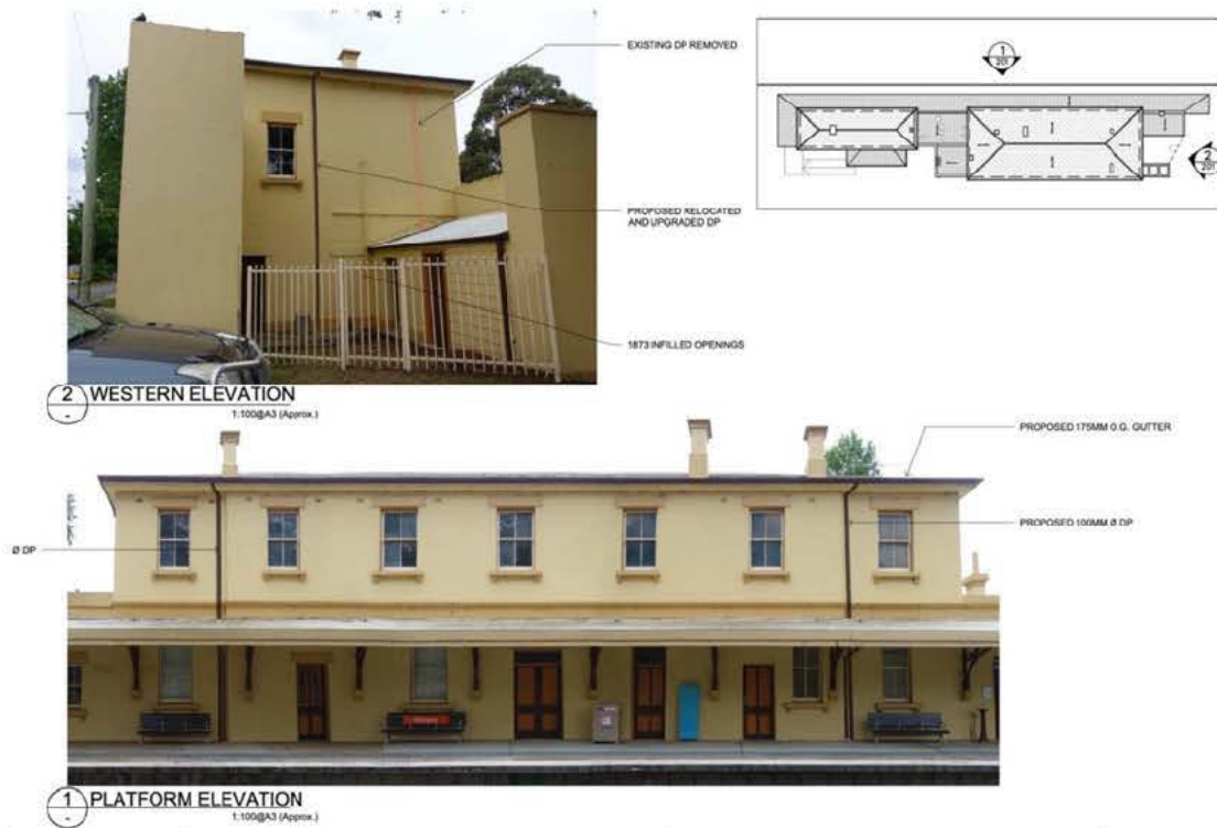
Figure 10 Photomontage showing proposed new downpipes to the platform and west elevations
