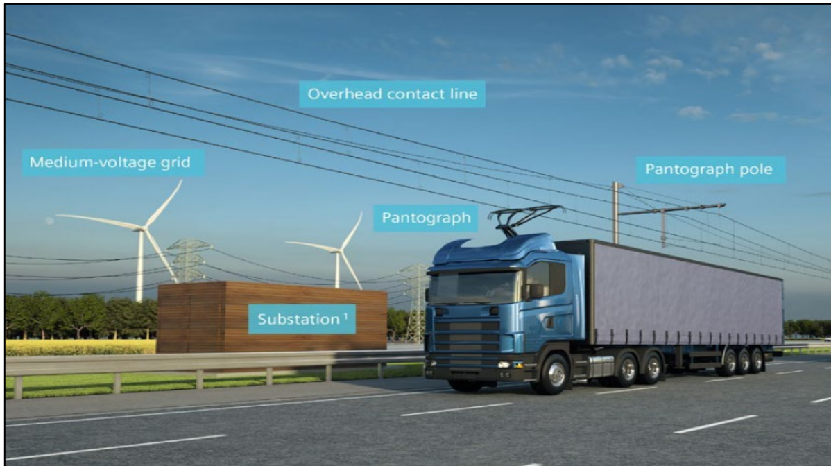
Figure 27: Siemens e-highway – overhead catenary electric road system
