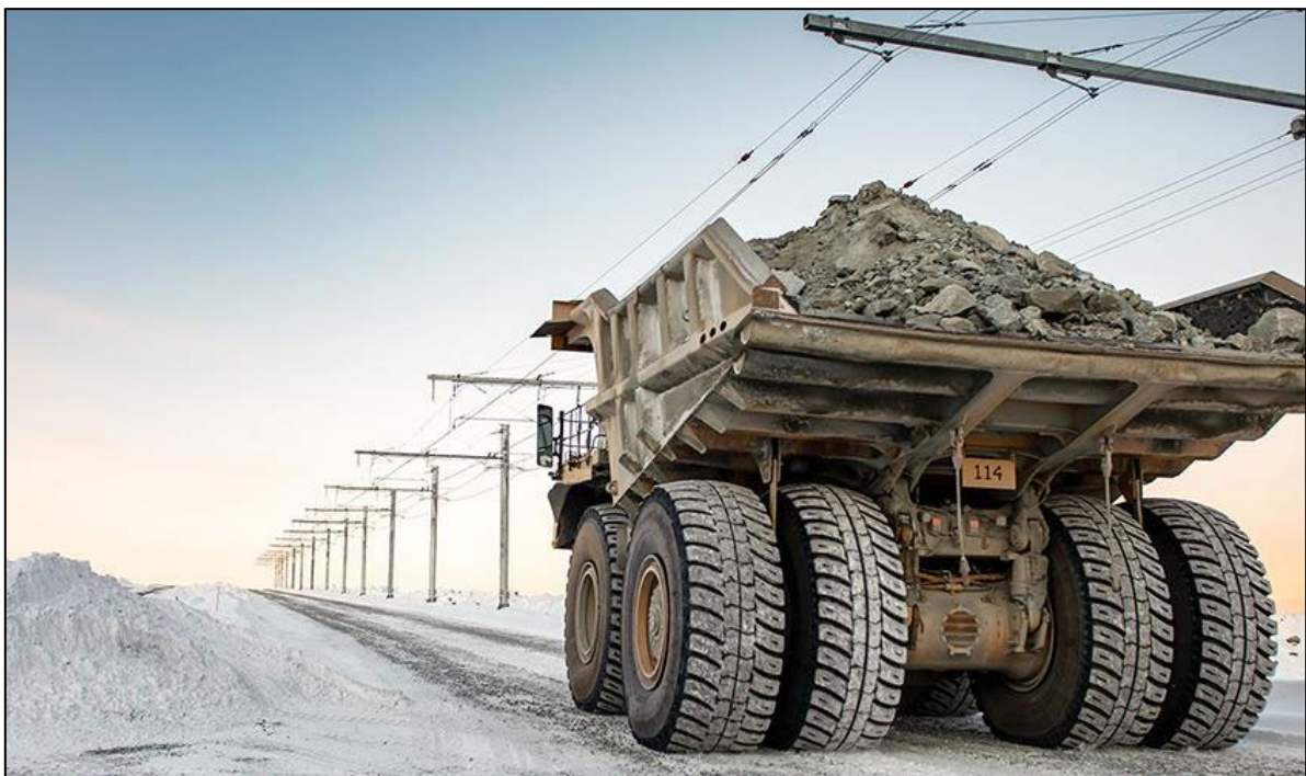
Figure 28: Mining truck using ABB's OCERS system at a mining site
