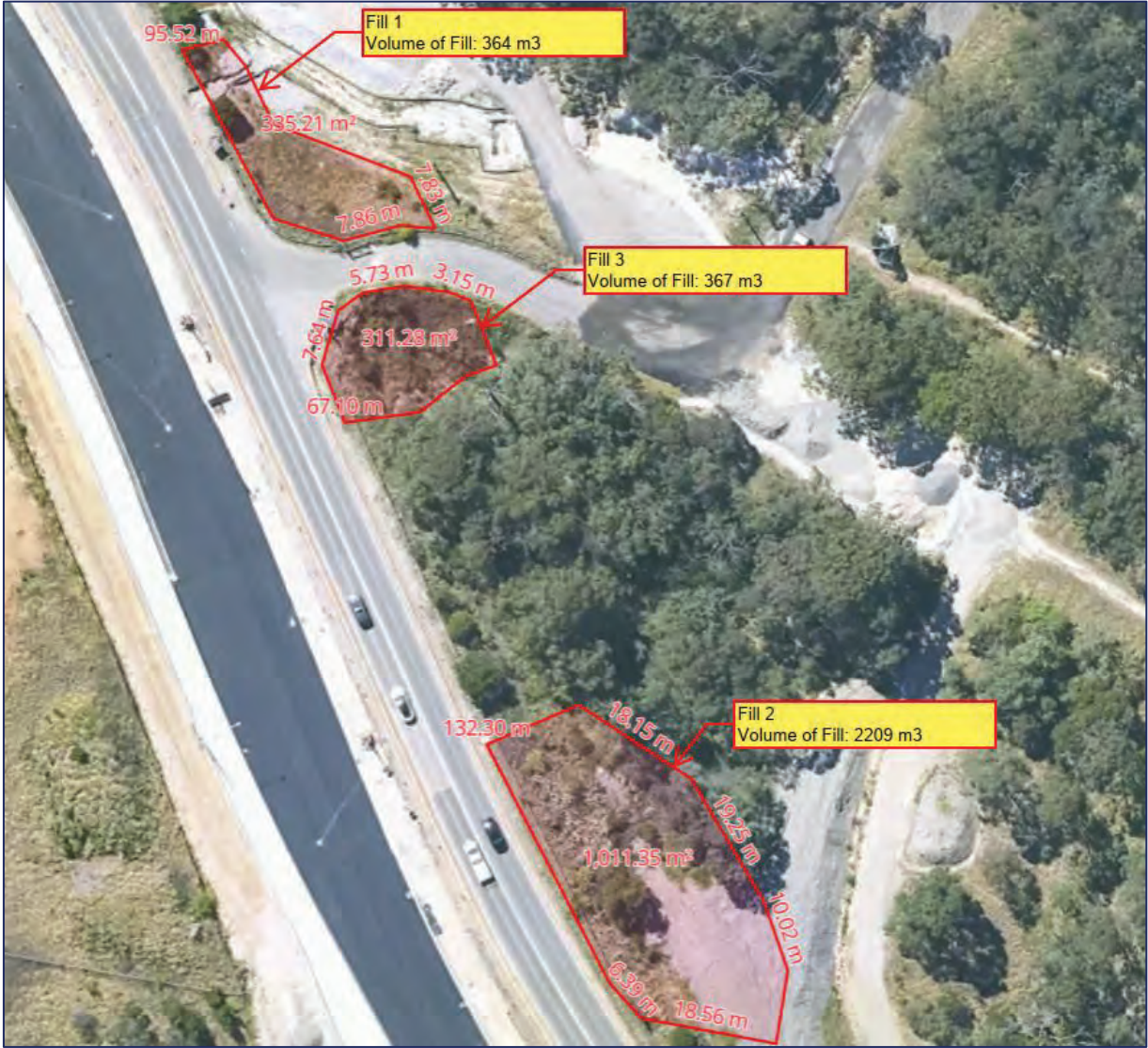
Figure 3-1: Key features of the fill emplacement sites.
