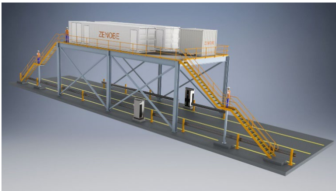
Figure 7 Visualisation of the proposed raised cable containment culvert and shipping containers above it.
