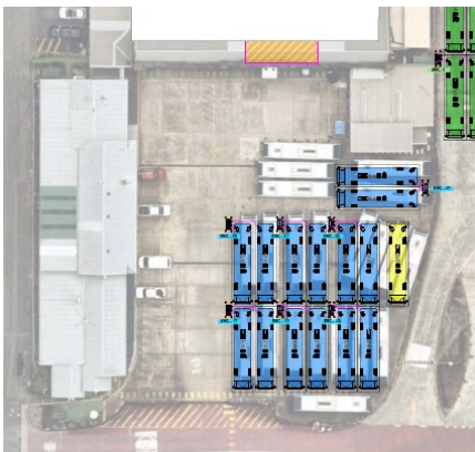
Figure 10 Detail of proposed Leichhardt Depot expansion showing the current proposed alignment of new chargers and buses in the former SRA office and amenities building
