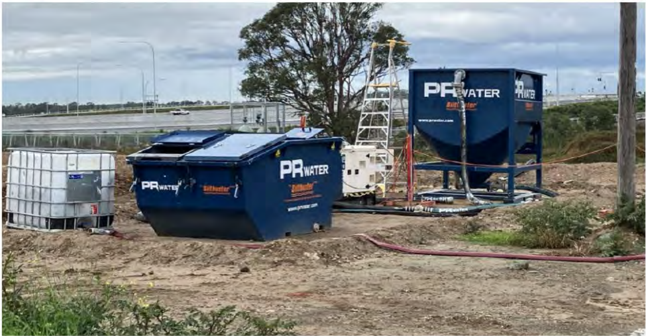
PR Water dosing unit which corrects pH in slurry prior to reuse.
