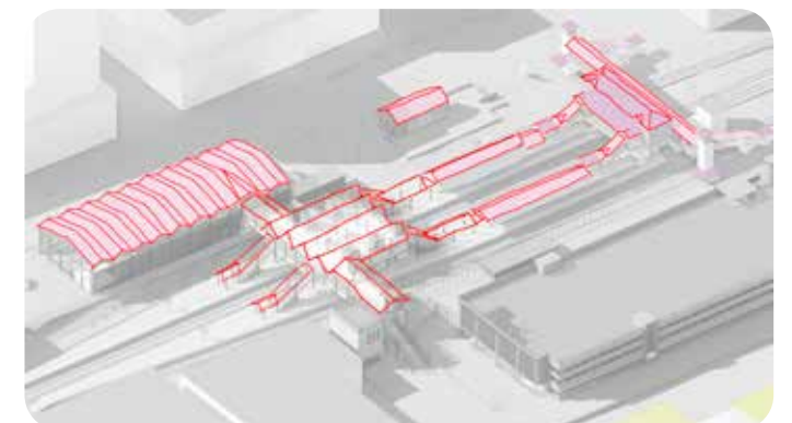
Figure 37: First pass at investigating the continuation of the station family aesthetic onto the Footbridge: a multi tier gabled roof.
