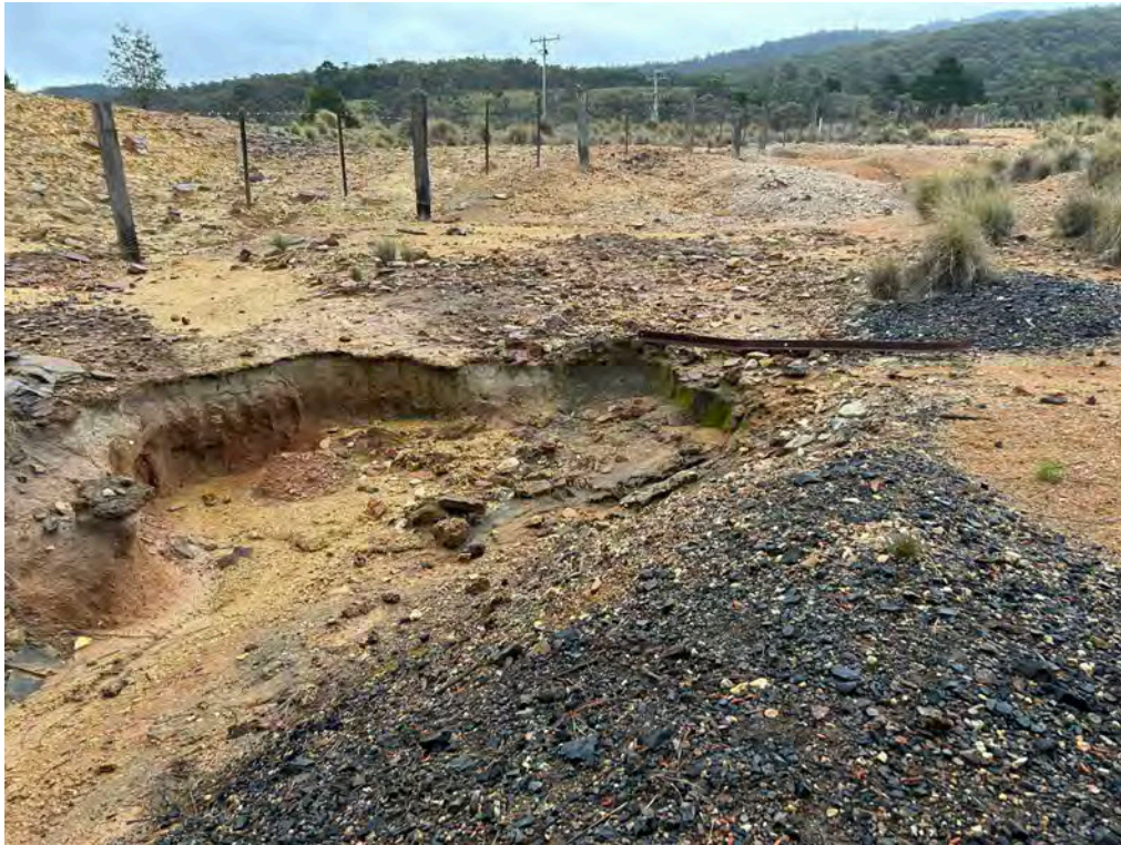
Photo 5: Evidence of erosion of soils on site observed during the previous inspections. Larger erosion has been observed during this inspection. No evidence of current surface water runoff into Coppers Creek was observed. Located south of the State Emergency Service (SES) facility.
