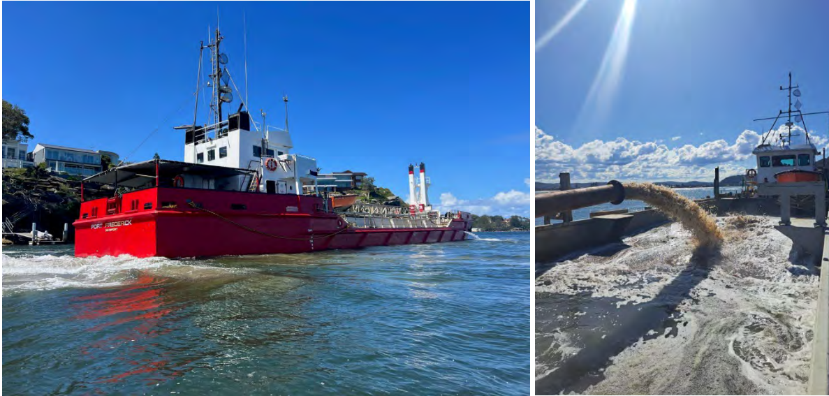
Figure 4-7: A TSHD vessel and hopper discharge (Source: McQuade Marine)
