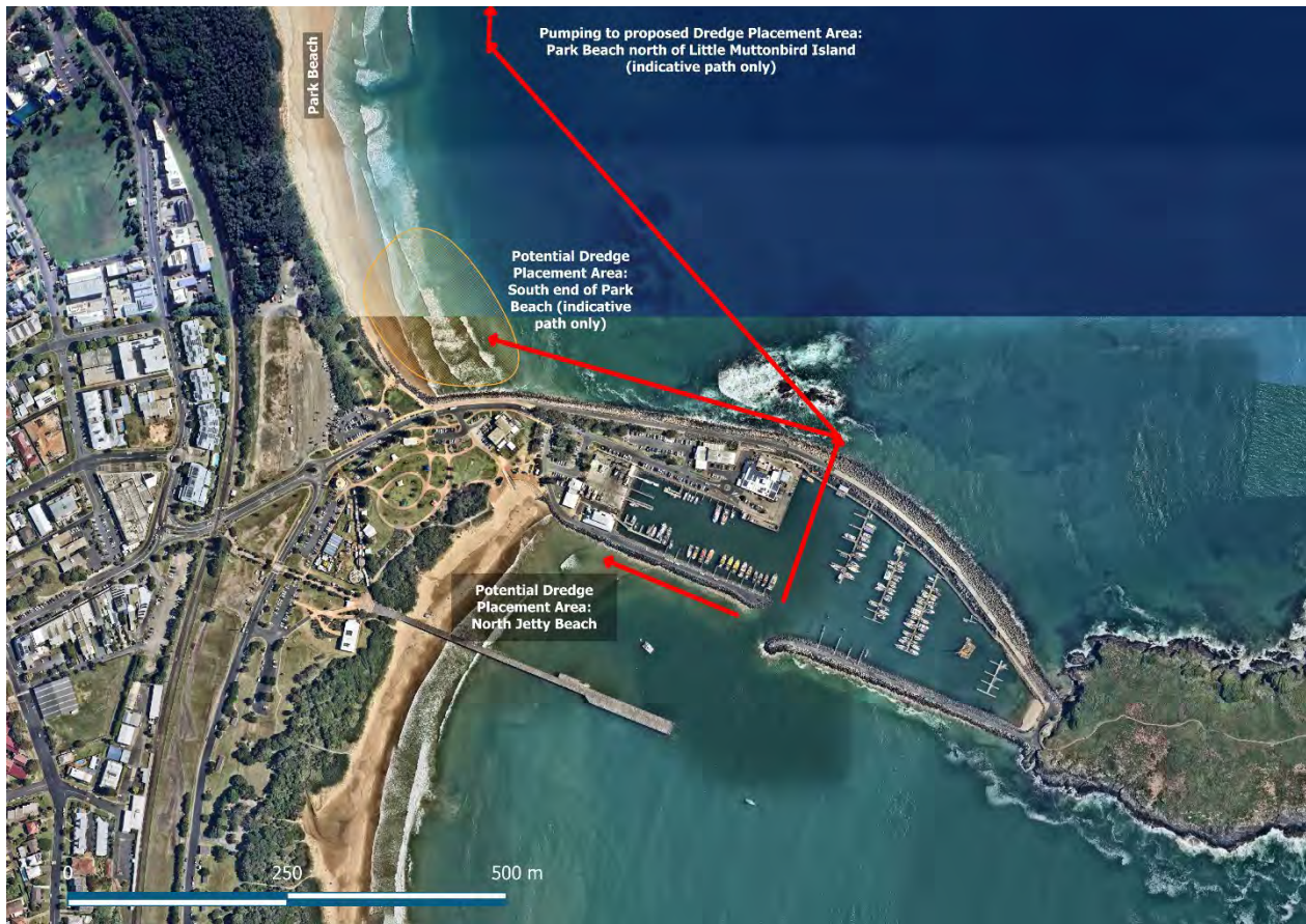
Figure 4-2: Pumping paths from Marina Entrance Channel
