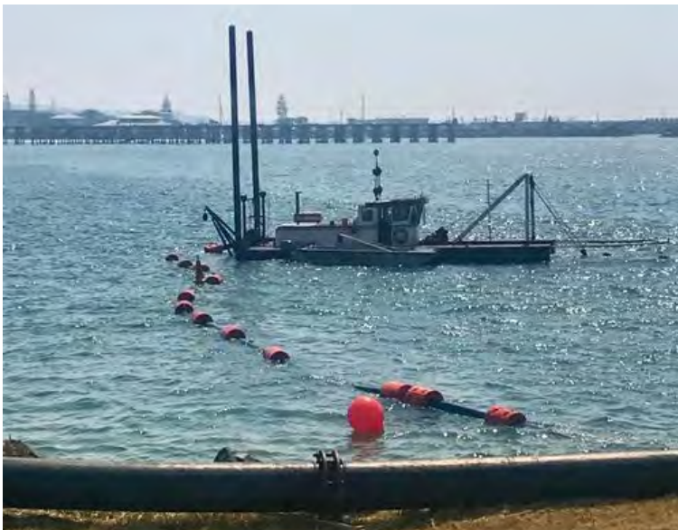
Figure 4-5: Small CSD and floating pipeline (Source: Maritime and Civil Group)
