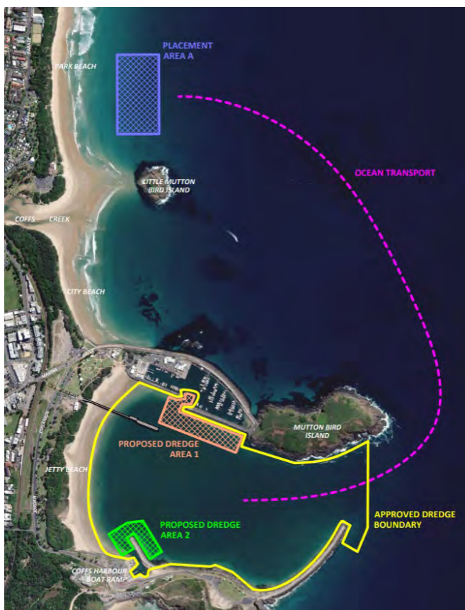
Figure 5-1: Preferred dredge transport option plan (North Coast Surveys, April 2024)
