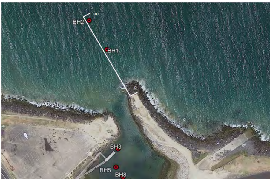
Figure 5-3: Borehole locations (Regional Geotechnical Solutions, 2020)
