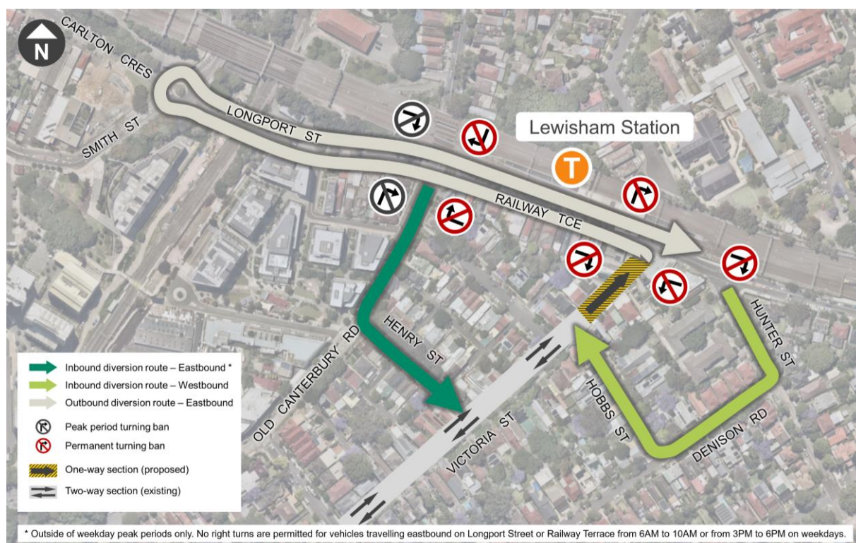
Figure 6-2: Diverted vehicle access routes to Victoria Street
