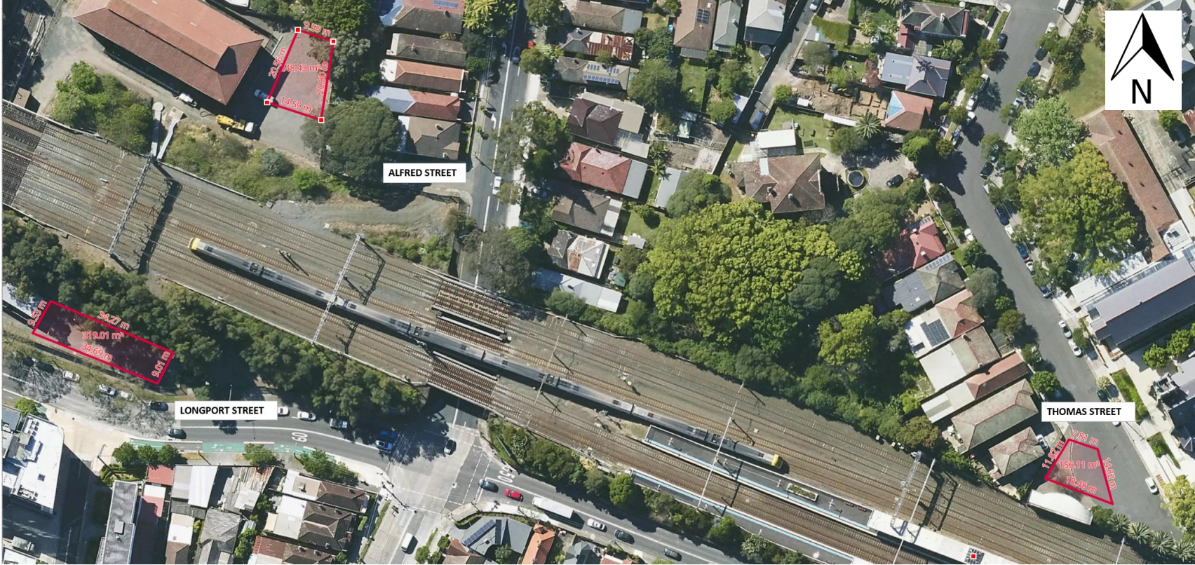
Figure 3-11: Proposed temporary construction compound areas
