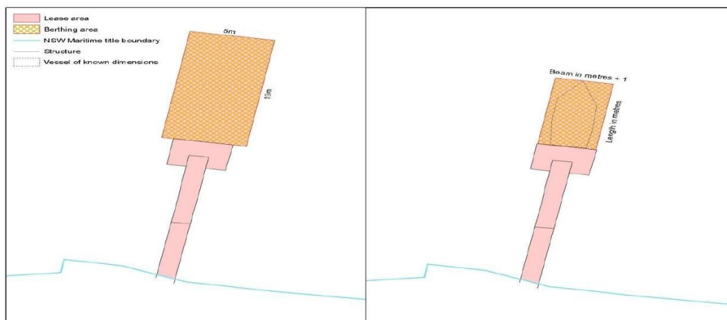
Figure 3 – Determination of the berthing area where a berthing facility is not delineated by mooring piles/blocks or where there are 2 piles only which are alongside the edge of the pontoon or similar structure
