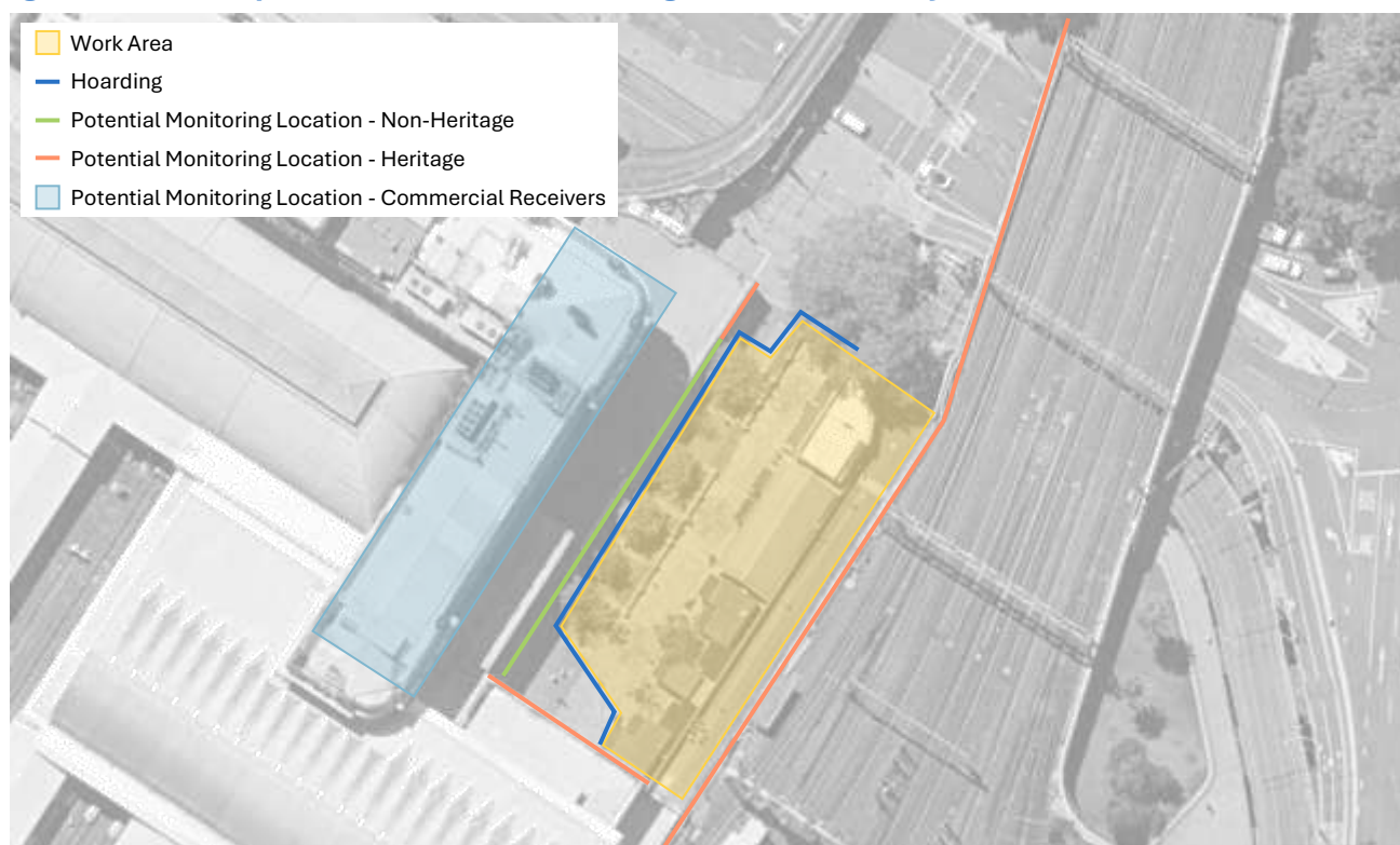
Figure 15 Proposed Vibration Monitoring Locations - Eddy Plaza
