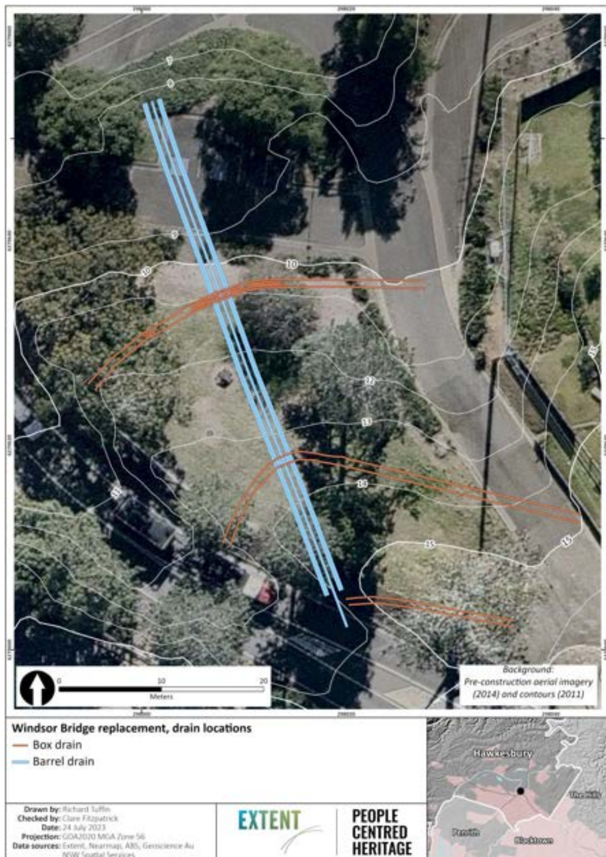
Figure 7-2 Pre-construction aerial photograph with contours showing drain locations.
