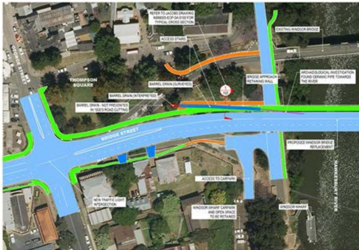
Figure 2: Image of the southern Windsor Proodge Replacement Project area with the location of the drain and its general course indicated. (Source: Jacobs 2018)
