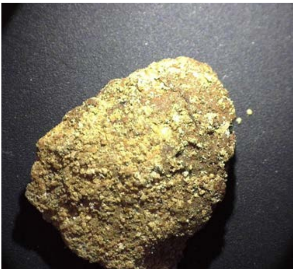
Figure 49 - Sample 2 of Patent cement. C.f with mortar. Note the larger consistent sand grain size (Source: AAJV 2018)
