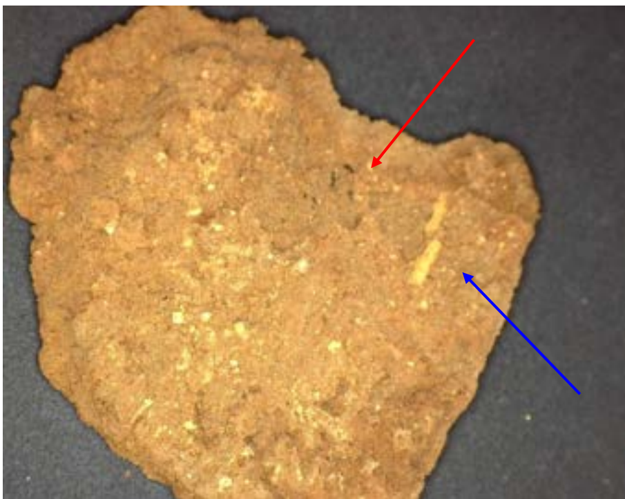
Figure 48 - Detail of Sample 1 mud mortar showing small charcoal fragments (red) and organic matter -sawdust/chaff (blue) inclusions. (Source: AAJV 2018)
