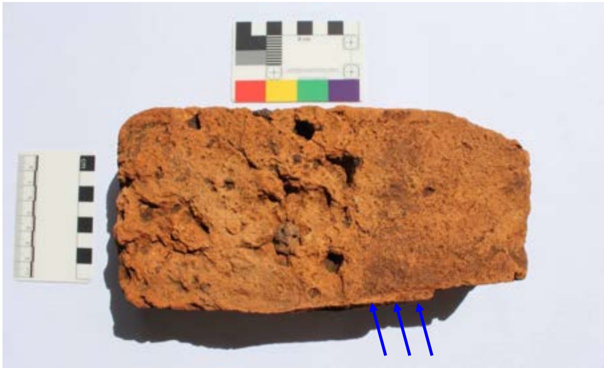
Figure 43 - Bed of sandstock Brick 1 from drain arch with cratered surface, probably from the expansion of water vapour during firing. Note the possible scribe line (indicated). (Source: AAJV 2018)
