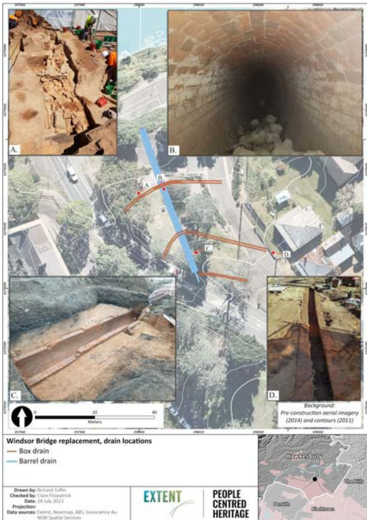
Figure 7-3 Pre-construction aerial photograph with contours showing drain locations with detail insets of the drain.
