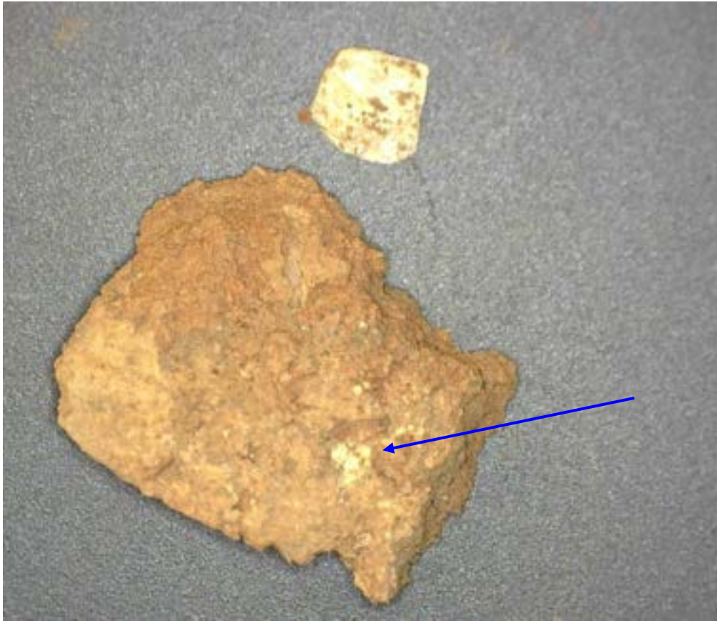
Figure 47 - Detail of Sample 1 mud mortar showing inclusion of calcined shell and larger calcined shell fragment. (Source: AAJV 2018)
