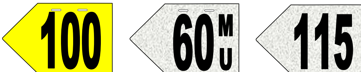
Figure 13 – Examples of pointed permanent track speed signs
