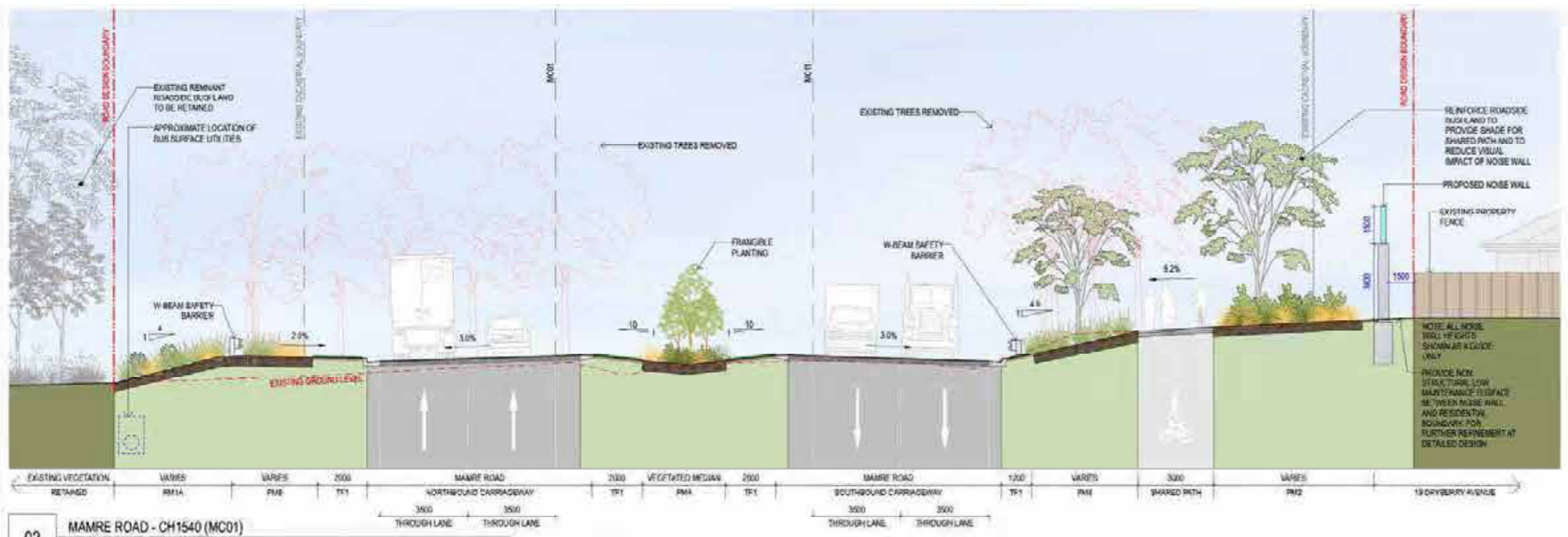
02 MAMRE ROAD - CH1540 (MC01) TYPICAL CROSS SECTION - SCALE 1:100
