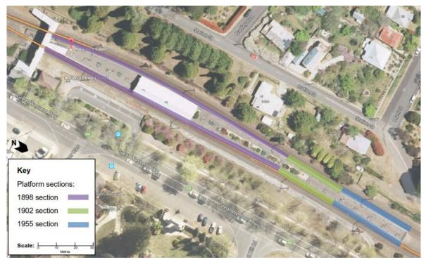
Figure 11 Plan sketch showing the changes in platform coping types (1898, 1902 and 1955)
