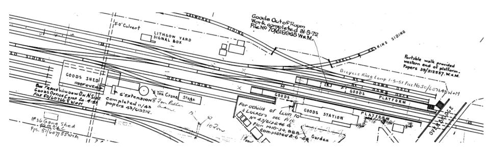
Figure 12: Detail of 1935 plan of Lithgow Goods Station (Eskbank Station); mark-up of structural changes provided post-1935. (Source: State Rail Archives CV-55771)
