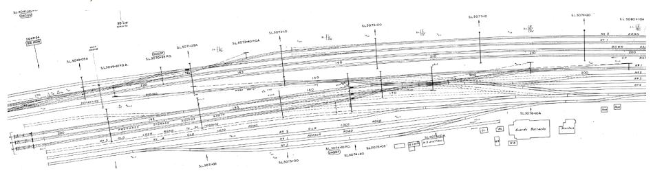
Figure 13: Detail of 1956 plan of area of former Eskbank Locomotive Depot, showing refuge and repair sidings. (Source: State Rail Archives CV-80604)
