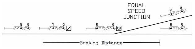
Fig 5.2 Equal Speed Junction - Signal at Stop
