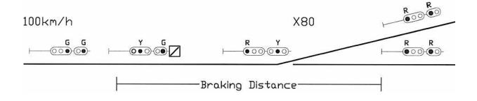
This is the result of a driver proceeding at turnout speed due to the display of the turnout repeater.
