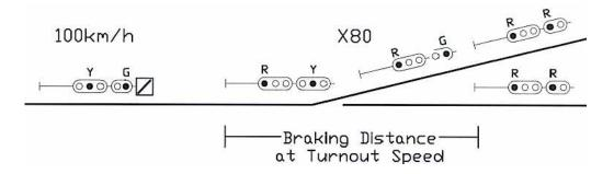
As the braking distance is adequate (in this example) from the turnout signal, then restricting this aspect to caution turnout provides a suitable solution.
