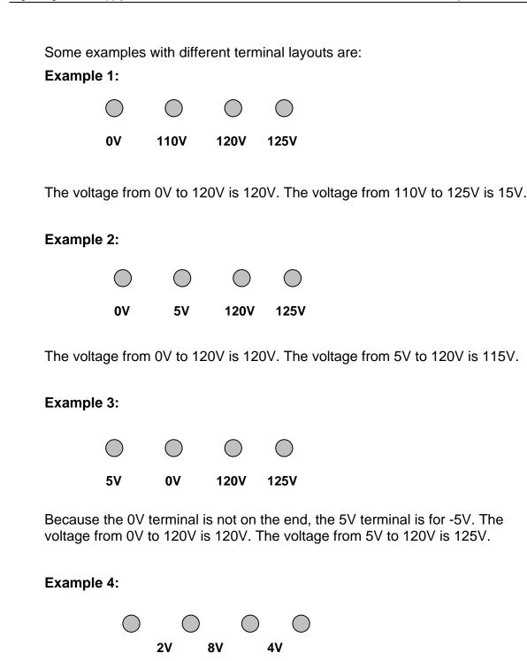
The voltage from the left of the 2V to the right of the 8V is 10V. The voltage from the left of the 8V to the right of the 4V is 12V. 4
