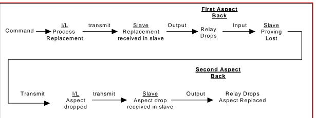
During this period an irregular aspect sequence may be observed if all signals were able to be seen together. However, the situation is safe as in the scenario of an aspect replacement, approach locking would hold the interlocking and is designed to specifically cover this situation.
