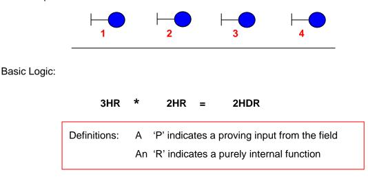
**Note**: It is considered that the HR (slave output) includes proving of the train stop reverse, hence VRR function does not need to be separately included.
