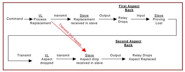
This diagram shows that the two aspects will now restore simultaneously.
