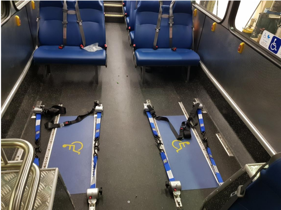
Image 2: One Door Urban Bus with seatbelts installed under the Program with the drop down seats removed. Note the lack of the stabilising back rest ('ironing board') and the wheelchair tethers located on the bus floor.
