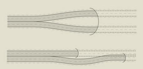
Figure 4.28 The top image reflects a double portal tunnel entry which tends to require a wider footprint. The bottom image illustrates a staggered portal arrangement that would limit the footprint width of the corridor to help reduce impacts to adjacent bushland areas
