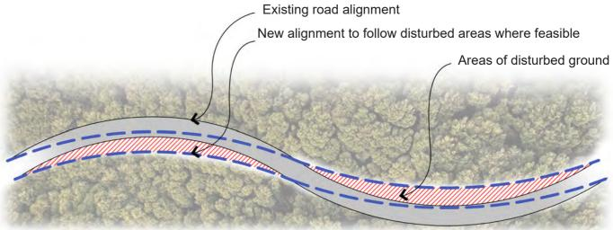
Figure 3.2 Alignment maximising disturbed areas
