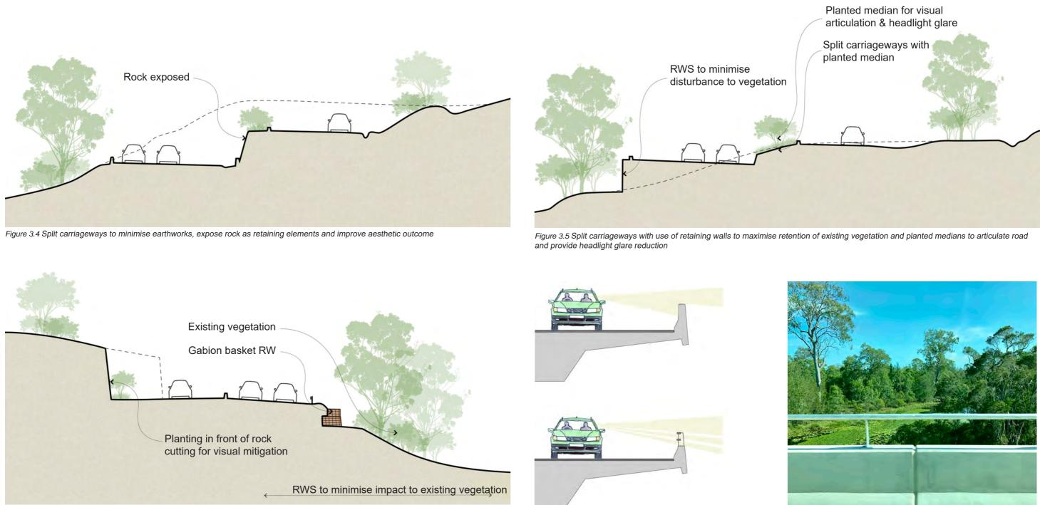
Figure 3.6 Planting in front of high rock cuttings and use of retaining walls to minimise earthworks to maximise retention of existing vegetation
