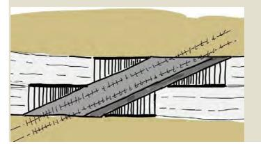
Figure 4.24 Plan view of a railway and highway crossing with a strong skew
