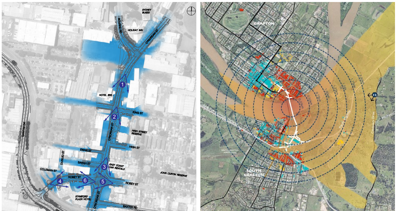
Figure 12 Examples of visual envelope maps, from the Sydney Airport North Precinct project and the Clarence River Crossing at Grafton
