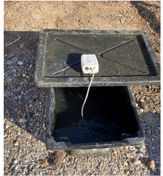
Figure 9.5: An aerated fish transport container. (Photo: Mathew Birch, Aquatic Science and Management)
